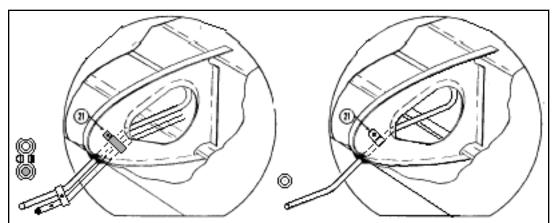
The original pitot-static booms were as shown on the left, with the pitot above the static tube, and clamped to each other. The front of the pitot tube was open, the front of the static tube closed, with small holes on each side. On the right, the later pitot design after the static port had been moved to the fuselage side.
