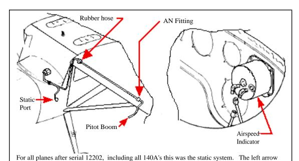
points to the static port forward of the left door and below the windshield. The pitot lines and pitot boom are noted. Note that the static line goes only to the airspeed indicator .
