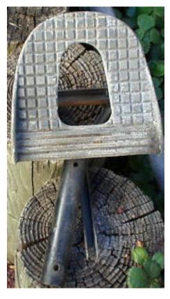
The pilot's side of the cast rudder pedal from a '46. This is an original, with no paint. Note the lack of any wear...this from the right side.
