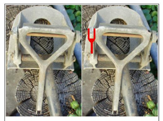
This is the front of the cast brake/rudder pedal from a '46 model.
