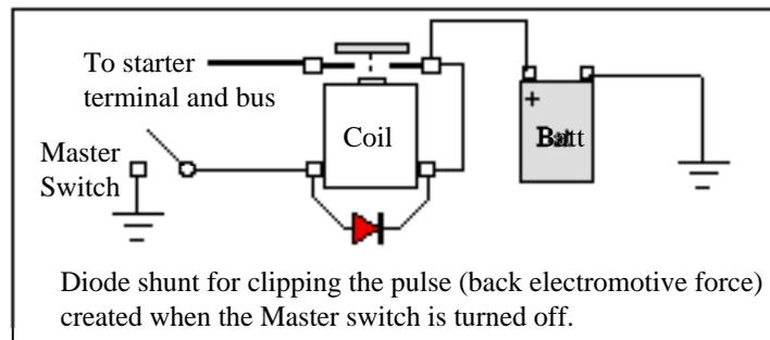
More and more planes are having the pull-style starter replaced by the electrically activated type via a relay. The reverse voltage pulse from the opening of the starter switch and the relay can be higher than for the battery solenoid, so Cessna also has called out for a diode to be in parallel with that coil, shown in the next sketch.
