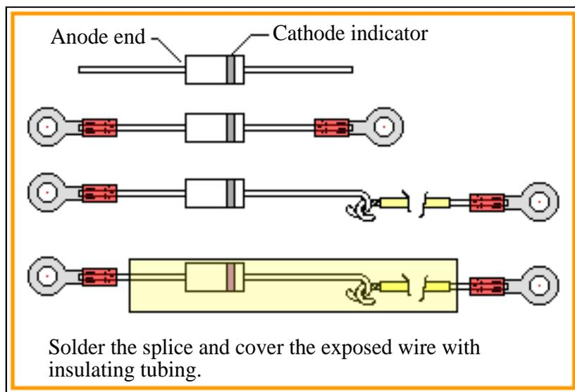
The polarity rule? The cathode (usually denoted by a contrasting color band at the cathode end) of the diode goes to the positive terminal of the coil, and the anode of the diode to the terminal where the wire to the master switch attaches. If you reverse this, the first time you turn on power will cause the diodes to smoke and their souls will depart this world. The acrid odor is unmistakable!
