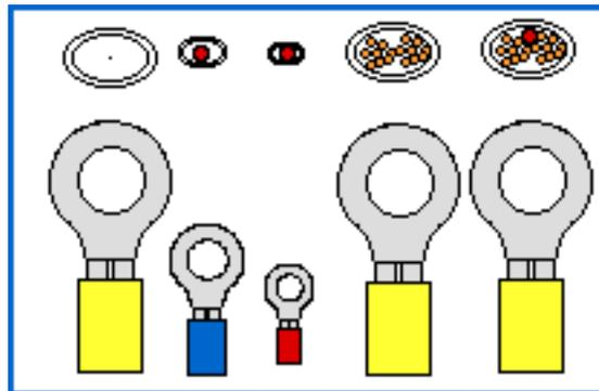
We found that Red or Blue terminals with the necessary 5/16ths hole are rare but even Radio Shack has yellow with 5/16ths hole as part of a package of various sizes. What is not well known is that you can use terminals which are grossly oversize for holding just the diode lead, shown as the red circle, if you fill up the excess opening in the yellow with more wire.
